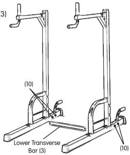
2. Secure the Upper Transverse Bar (4) to the 2 Support Bars (2) with four M10x60 Bolts (10).
