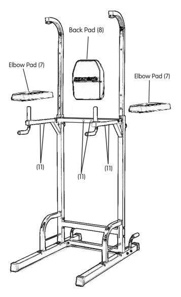
1. Place the Pull-up Bar (9) to the two Upper Elbow Bars (6) and tighten using the two Knobs and Carriage Bolts (13).
